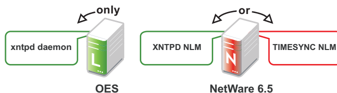
Figure 10-1 Time Synchronization for Linux and NetWare
